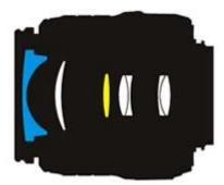
Aspherical lens elementsED glass elements E: Super ED glass elements
