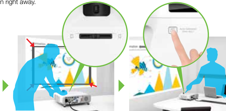
Keystone correction with Horizontal Keystone Adjuster & Auto Vertical Keystone
