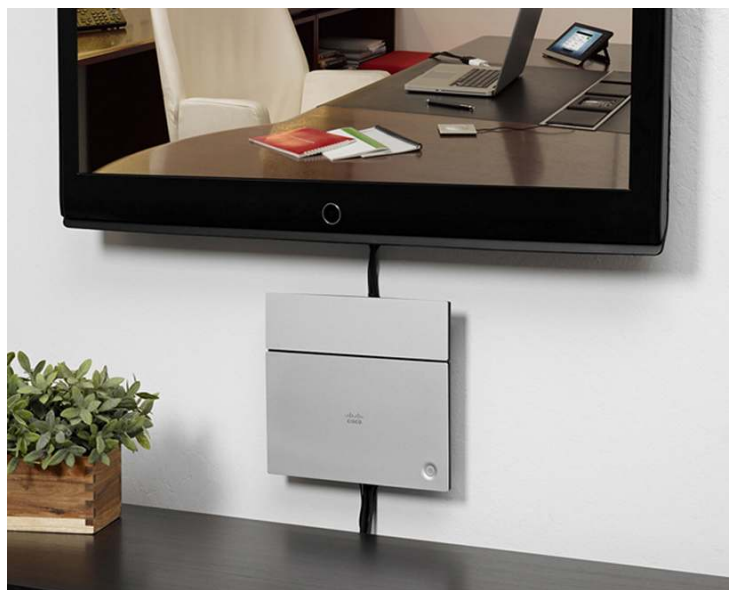
Figure 3. Cisco TelePresence SX20 Quick Set on Wall Mount
